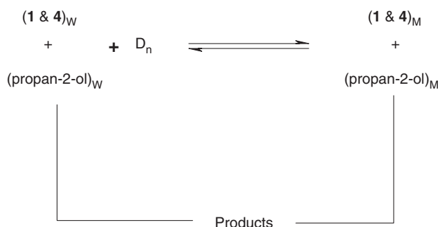
Scheme 3. Partitioning of the reactive species between the aqueous and micellar phase.
